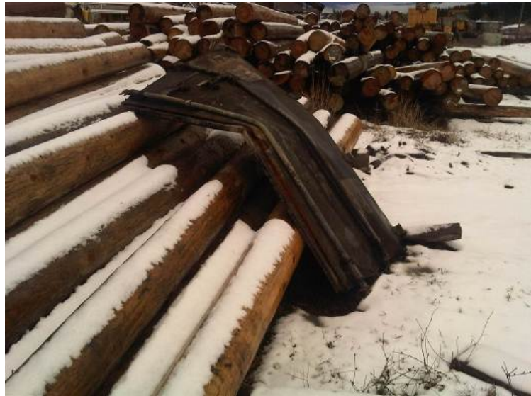
The photo above shows the bending of one of the container doors that was blown off in the explosion.
